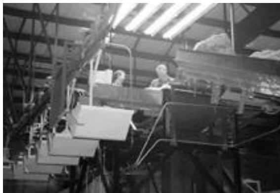
This shows the grading table where all wool is individually fleece graded. Twenty-four different grades of wool are made in the Mid-States warehouse in Ohio. In addition, custom blends to customer specs can be made up in 45,000 pound units.
